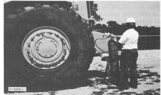
CORRECT POSITION FOR TIRE INFLATION (Behind the Tread)
